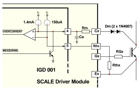
Fig. 4 Collector-sense circuit principle
