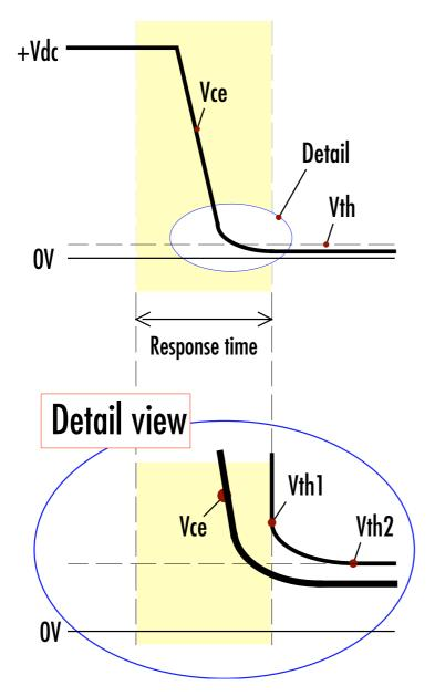
Fig. 5 Collector-sense voltage curve
